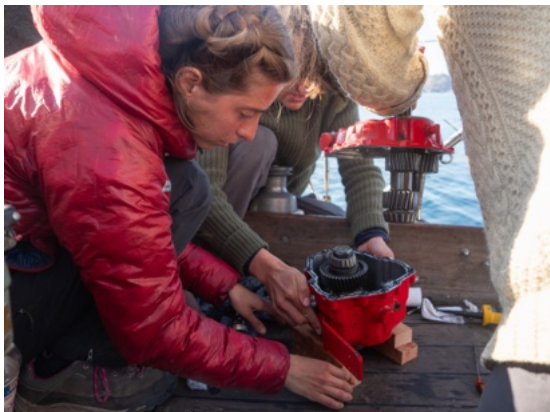
Resealing the gearbox.
